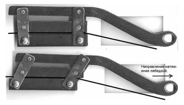
A winch is attached to the hole in the tool and placed by the place where the guy is fastened.
